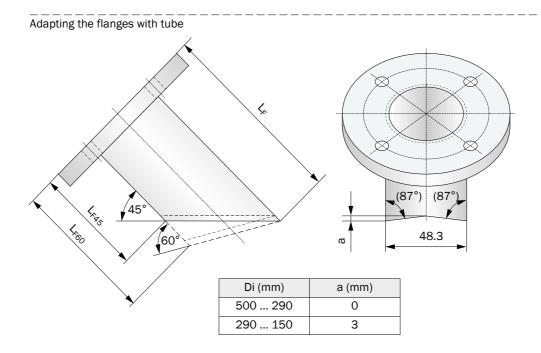
Flange tube length L<sub>F</sub> (L<sub>F45</sub>, L<sub>F60</sub>) depends on installation angle  $\alpha$ , wall thickness w and nominal length NL ( $\rightarrow$  Fig. 22,  $\rightarrow$  Fig. 23). This correlation is expressed by the following formulas:
