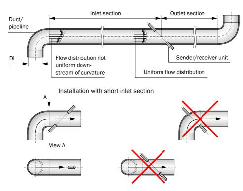
Installation with inlet and outlet sections of sufficient length
