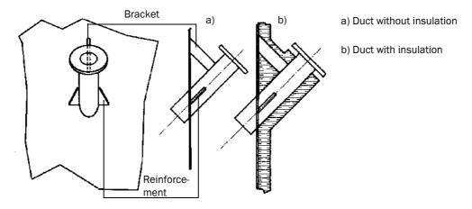
Flange with tube mounted on brick or concrete duct
