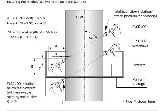
Select an installation angle of  $60^\circ$  for duct diameters as from approx. 4.5 m.
