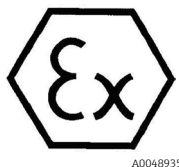
Figure 3. ATEX label for use in hazardous areas
