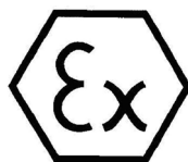
Figure 4. ATEX label for use in hazardous areas
