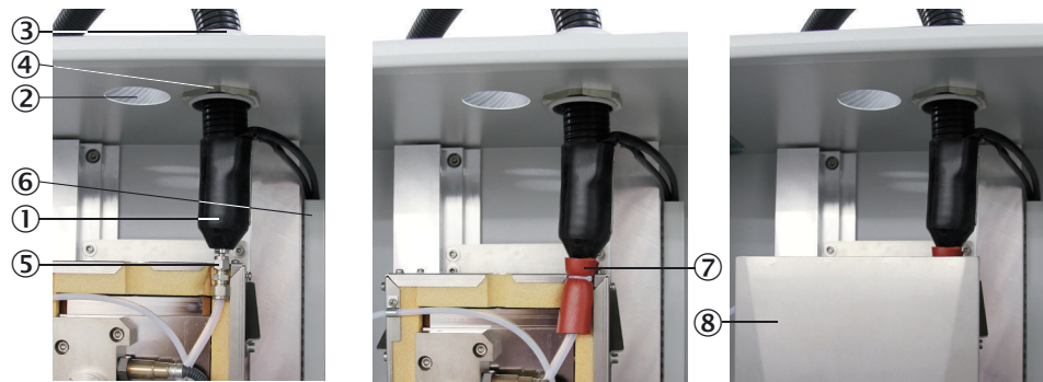
Figure 8: Sample gas line - connection diagram
