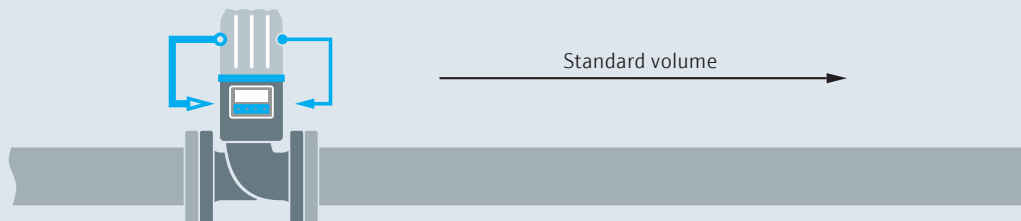
Gas flow meter with volume corrector and internal p/T sensor
