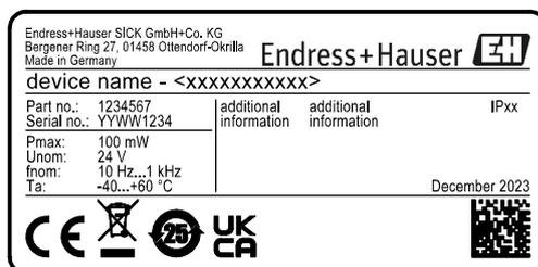
Figure 3: Analyzer type plate, schematic representation
