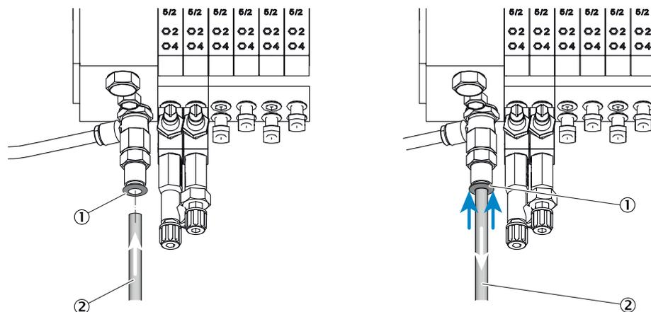
Figure 5: Push-in fitting with retaining ring (example shown)
