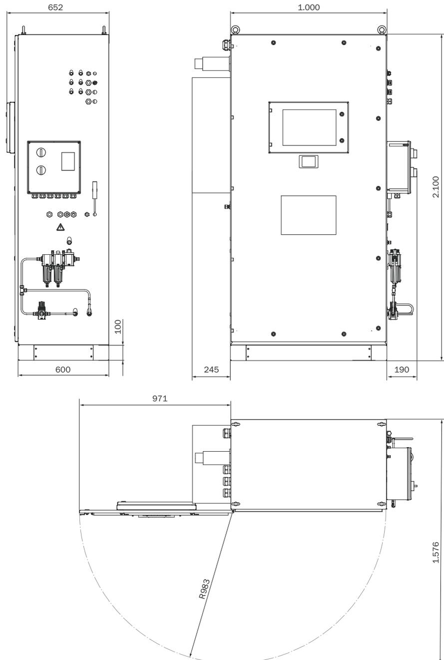
Figure 10: MCS200HW Ex p (dimensions in mm)
