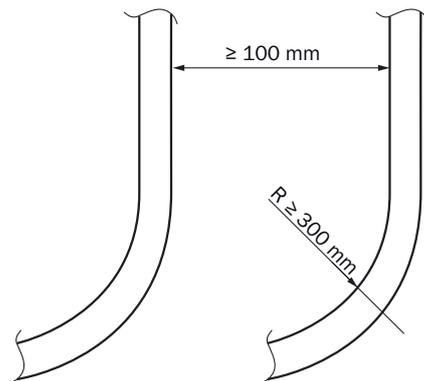
Figure 6: Lines – clearance and bending radius
