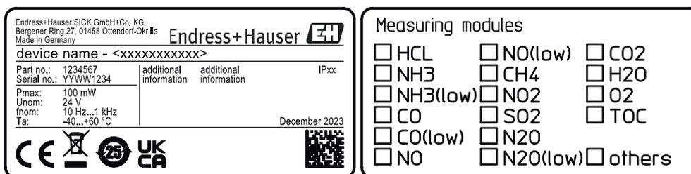
Figure 2: Type plate of complete device, schematic representation
