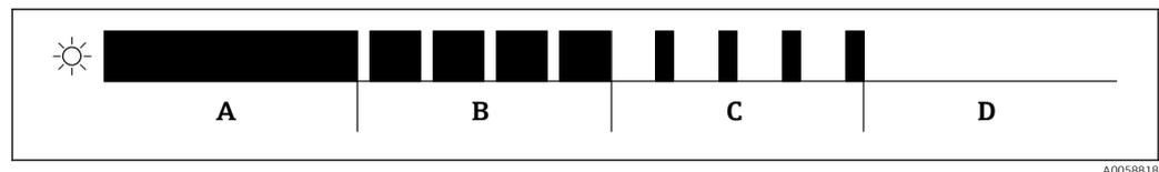
17 Graphic display of different flashing states of the LEDs when a function is selected
