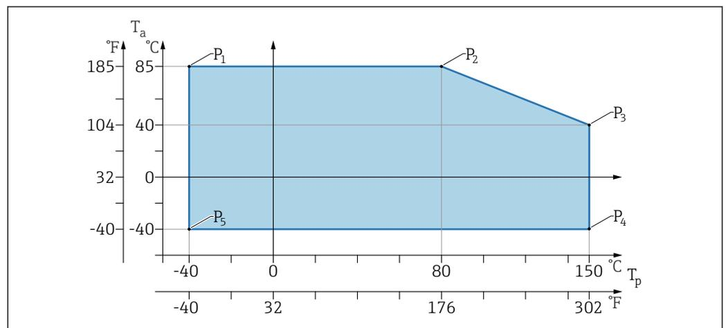
22 Ambient temperature  $T_a$  depending on the process temperature  $T_p$
