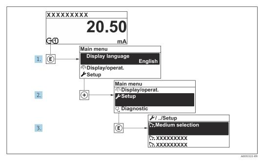
Navigation to the "Setup" menu using the example of the local display
