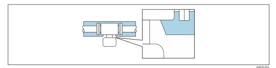
$\blacksquare$  6 Thermal insulation with exposed extension neck
