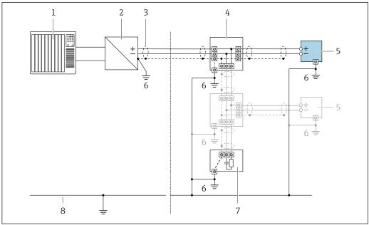
■ 10 Connection example for FOUNDATION Fieldbus
