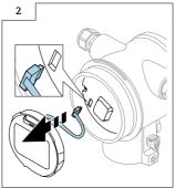
► Press the release mechanism and remove the display module.
