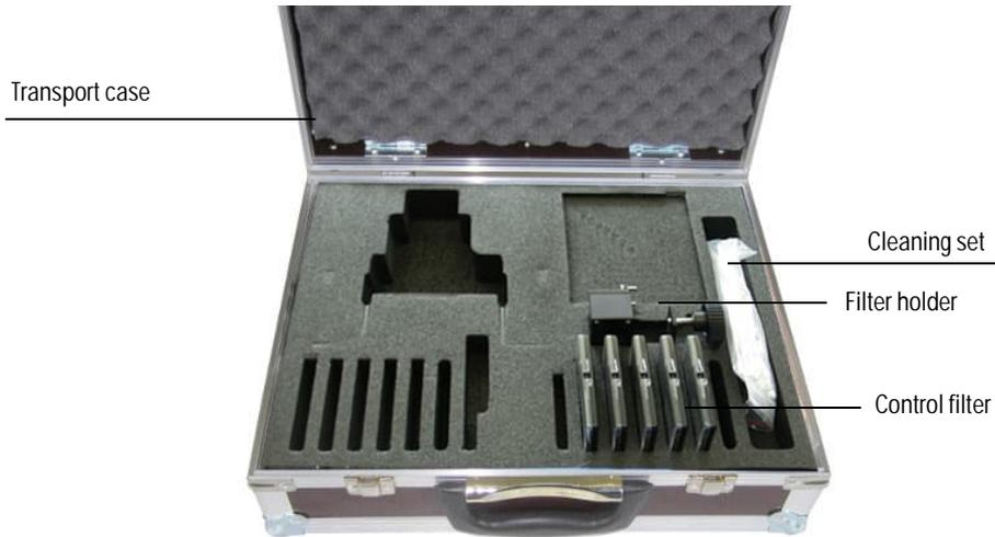
Fig. 21: Components of the equipment for the linearity test
