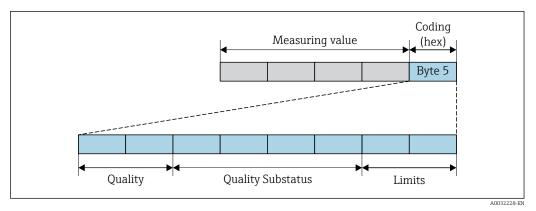
■ 30 Structure of the coding byte
