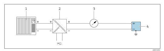
2 12 Connection example for 4 to 20 mA current output (passive)
