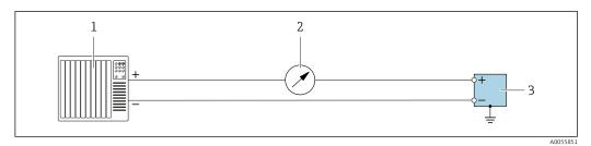
■ 11 Connection example for 4 to 20 mA current output (active)
