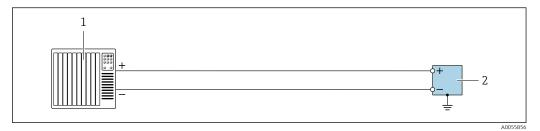
Connection example for pulse output/frequency output/switch output (active)
