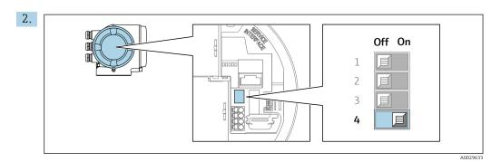
To switch addressing from software addressing to hardware addressing: set the DIP switch to **On**.
