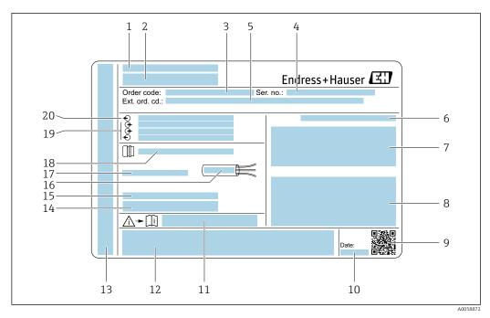
■ 2 Example of a transmitter nameplate
