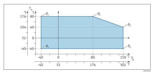
$\blacksquare$  11 Ambient temperature  $T_a$  depending on the process temperature  $T_p$
