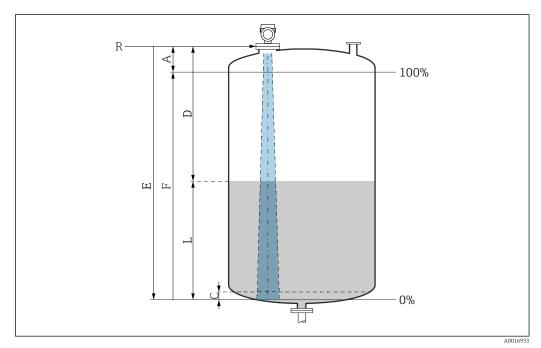
Configuration parameters for level measurement in liquids
