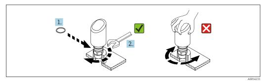
■ 2 Screwing in the device
