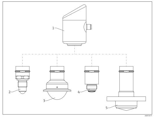
■ 1 Product design Micropilot FMR43 with sample process connections
