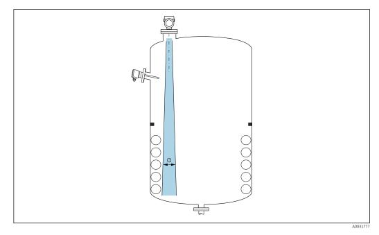
Avoid internal fittings (level switches, temperature sensors, struts, vacuum rings, heating coils, baffles etc.) inside the signal beam. Pay attention to the beam angle  $\alpha$ .
