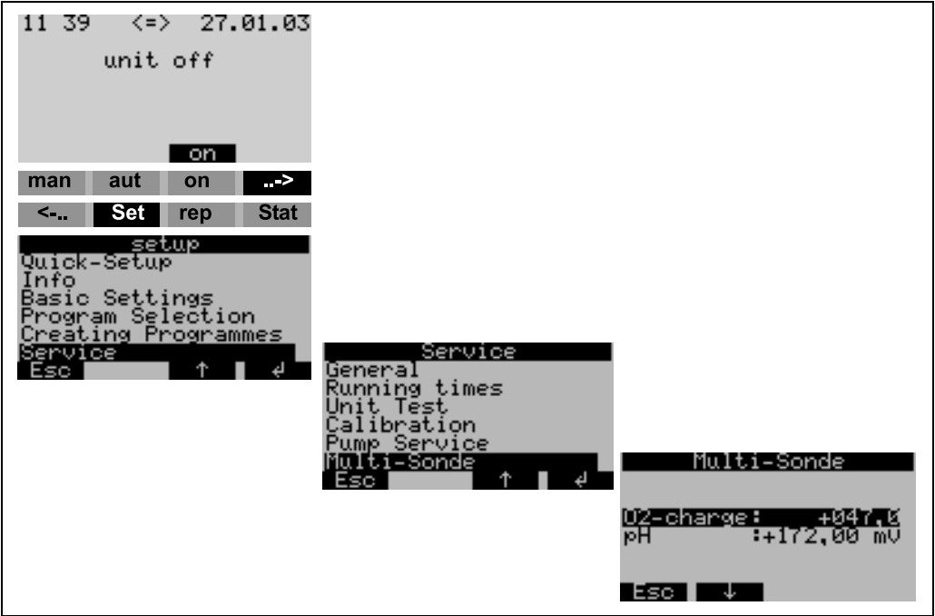
Fig. 21: Checking pH measurement (Sensor Check System)
