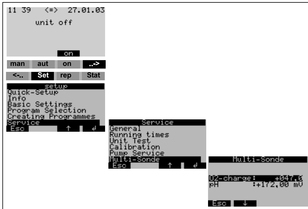
Fig. 22: Checking oxygen measurement (Sensor Check System)
