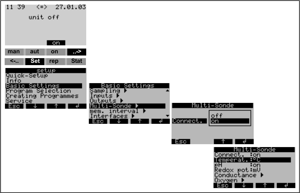
Fig. 23: Commissioning the multi-parameter probe (optional)
