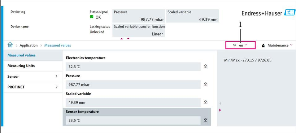
The screenshot shows the 'Measured values' page in the Endress+Hauser web interface. The page displays various sensor readings and their units. A language dropdown menu is highlighted with a red box and labeled '1'.
