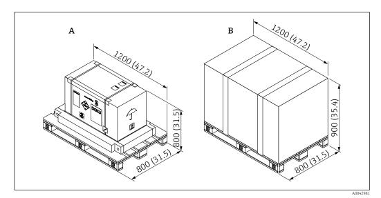
🖻 1 Dimensions of packaging kit (71341833). Unit of measurement mm (in)
