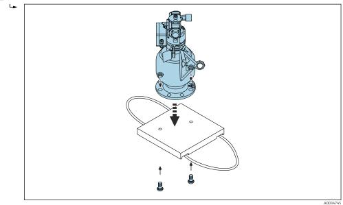
2. Use the short harness to secure the top of the source container that is attached to the base plate in order to guard against tipping when lifted.
