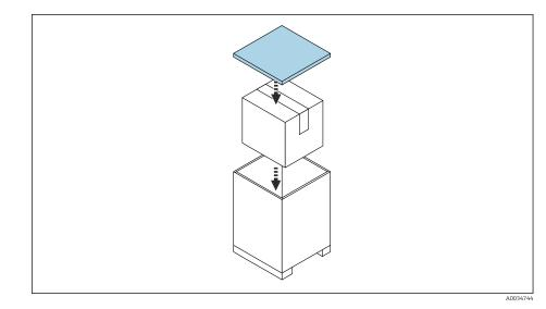
5. I Mark the seaworthy overpack as a Type A package. Mark the cardboard box as the overpack of a Type A package.
