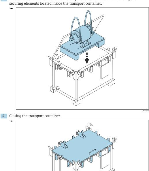
**3.** Place the source container into the transport container and secure it using the securing elements located inside the transport container.
