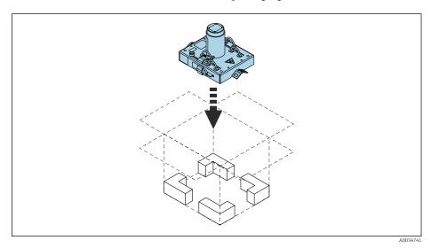
2. Apply the labeling kit provided to the source container in accordance with the applicable IATA requirements and national regulations. Secure the source container using packaging foam pieces.
