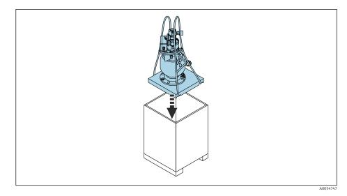
4. Secure the source container using packaging foam pieces.
