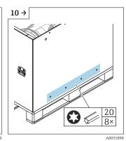
Screw the lower wood screws into the long sides in the wooden crate
