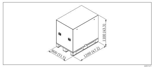
2 Overpack for loaded or unloaded source containers, dimensions of packaging kit (71697741). Unit of measurement mm (in)
