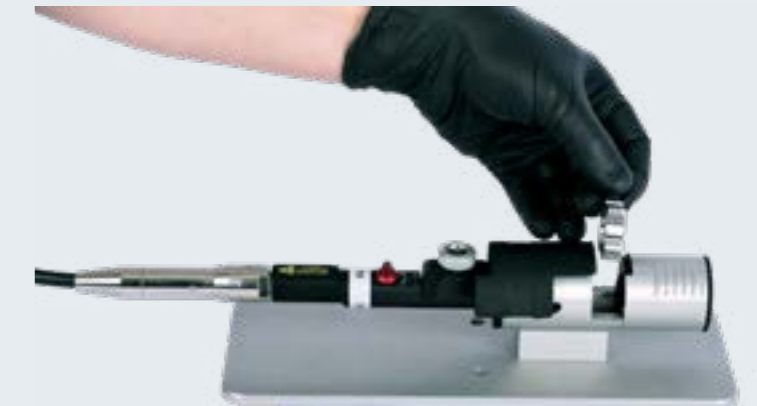
A verification cell being inserted into a micro flow bench connected to an Rxn-10 probe
