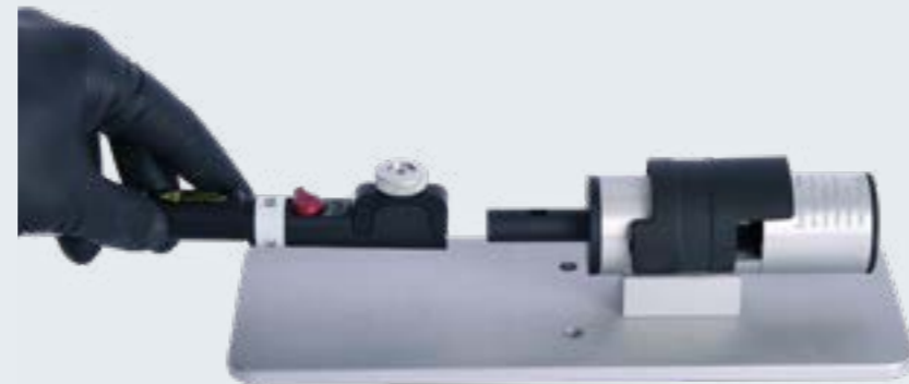
Connecting the Raman Rxn-10 probe to the micro flow bench
