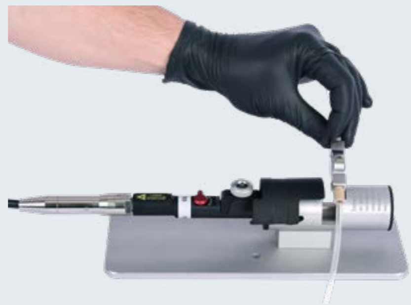
Inserting the micro flow cell into the micro flow bench
