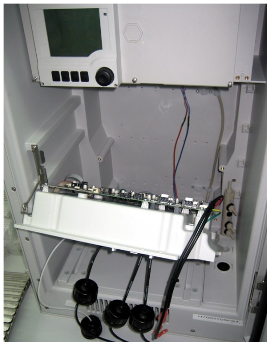
Figure 3: Mounting plate, popped out and fixed
