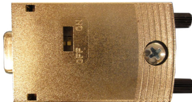
Fig. 10: Plug with slide switch for terminating resistor
