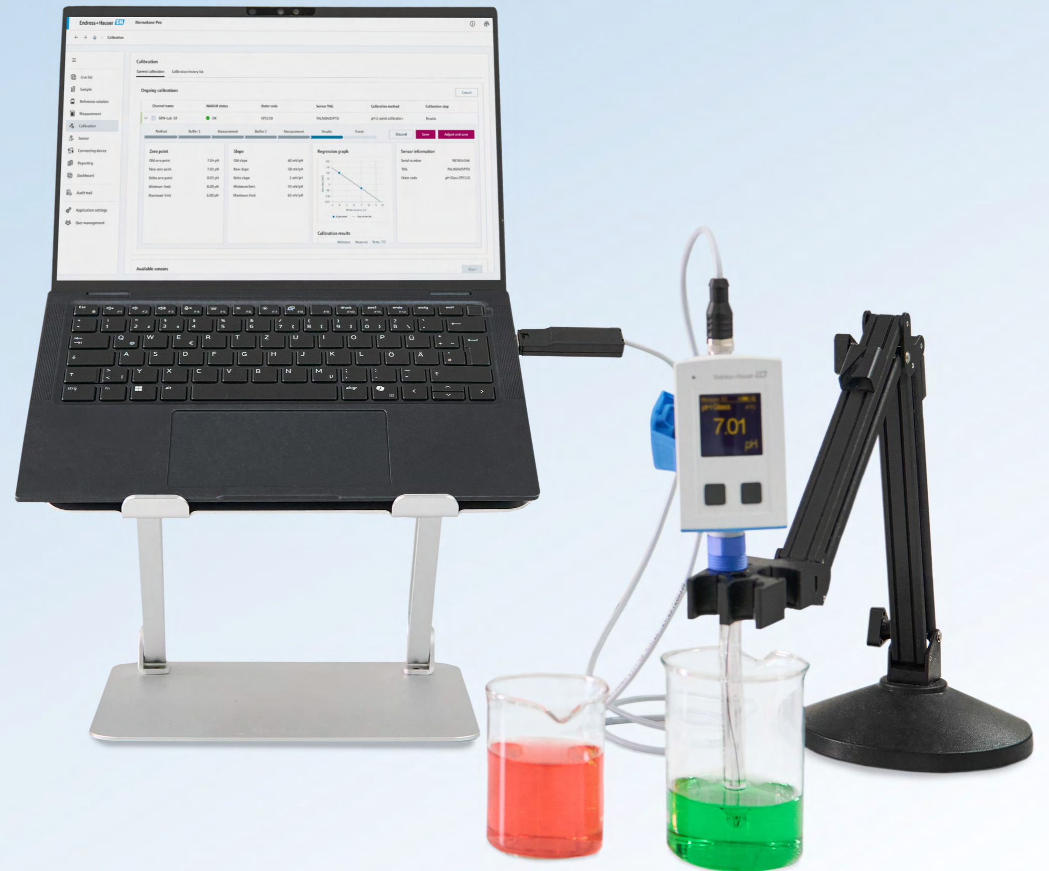
Memobase Pro software with Liquiline CML18 and pH measurement
