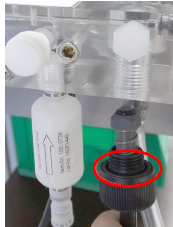
O-ring for alkalization unit or for overflow valve/pressure limiter of sample condit. unit (outside)
