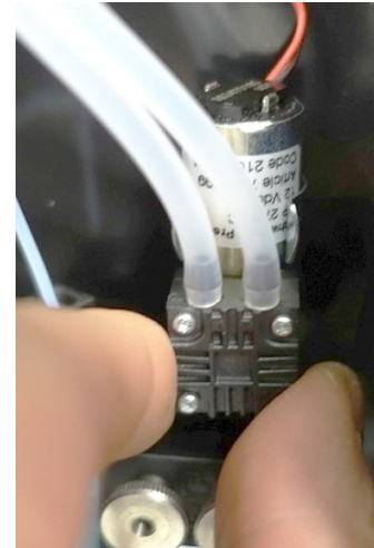
Figure 17: Removal of alkalization pump
