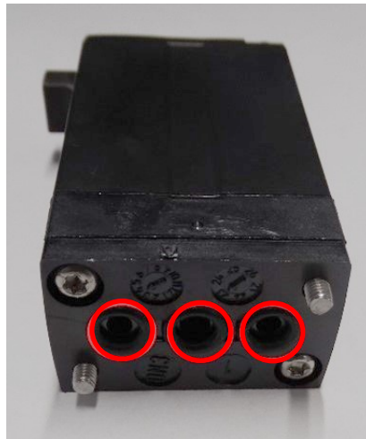
O-rings for valves of the sample conditioning unit
