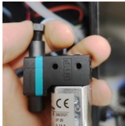
Figure 19: Removal of the circulation pump
