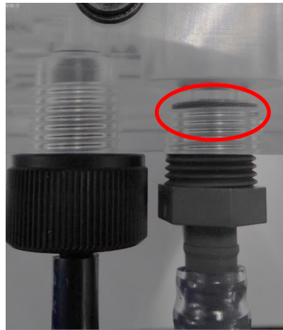
O-ring for drain of sample conditioning unit
