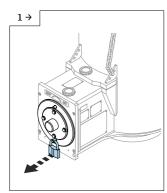
Remove the lock on the shutter cover and store it safely.
