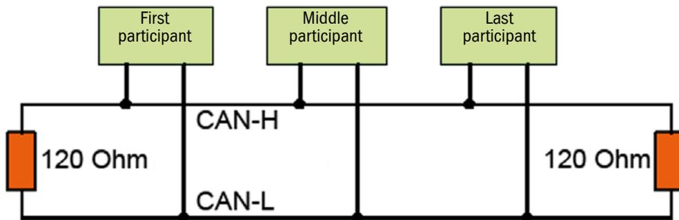
Terminating resistors must be activated for first and last bus participants.
