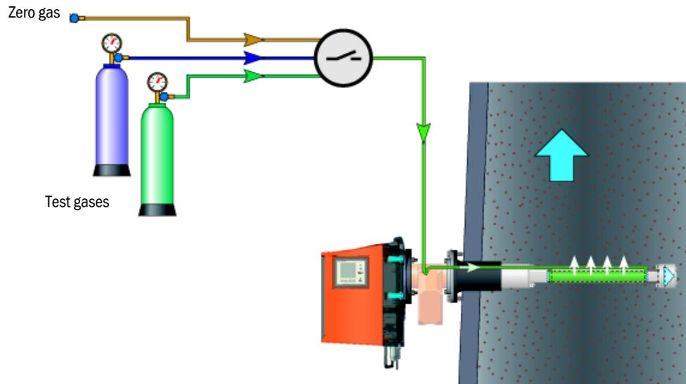
For GPP measuring probes, a gas check can be carried out with the measuring probe fitted in the gas duct.
