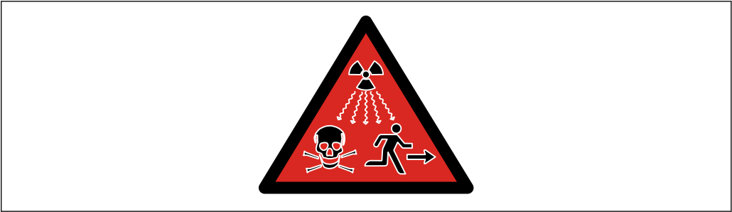
1 Warning symbol for highly radioactive source according to ISO 21482
