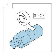
Only required if the vent valve not pre-assembled with PTFE sealing tape.
