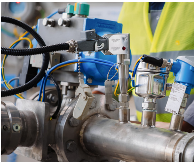
Left to right: Endress+Hauser Raman Rxn-40 probe, Liquiphant FTL50 point level switch, and iTHERM ModuLine TM131 thermometer
