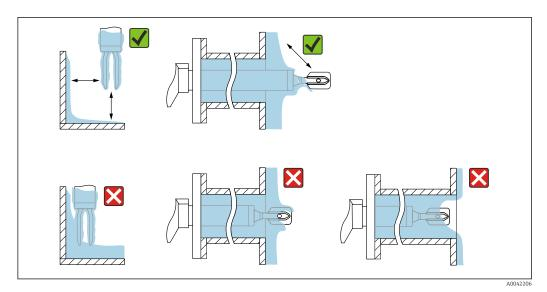
$\blacksquare$  9 Installation examples for a highly viscous process medium
