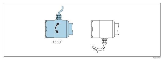
■ 14 Housing without locking screw with drip loop
