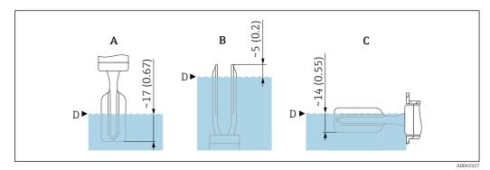
$\blacksquare$  6 Typical switch points, enamel-coated tuning fork. Unit of measurement mm (in)
