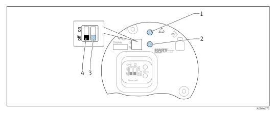
$\blacksquare$  27 Operating keys and DIP switch on FEL60H electronic insert
