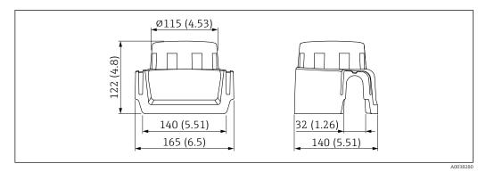
■ 31 Protective cover for aluminum single compartment housing. Unit of measurement mm (in)
