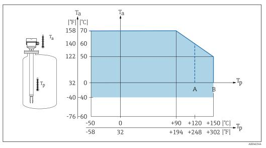
$\blacksquare$  33 Permitted ambient temperature  $T_a$  at the housing as a function of the process temperature  $T_p$  in the vessel
