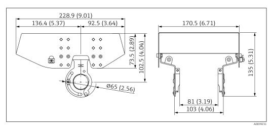
■ 30 Weather protection cover for dual compartment housing. Unit of measurement mm (in)
