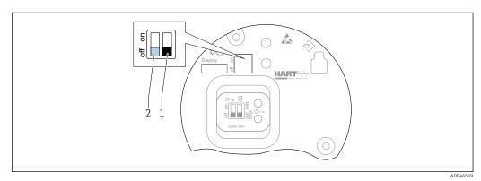
■ 28 Functions of DIP switches on the FEL60H electronic insert
