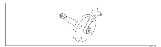
Position of the tuning fork when installed horizontally in the vessel using the marking
