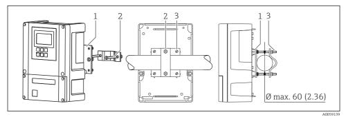
Mounting on horizontal or vertical pipes
