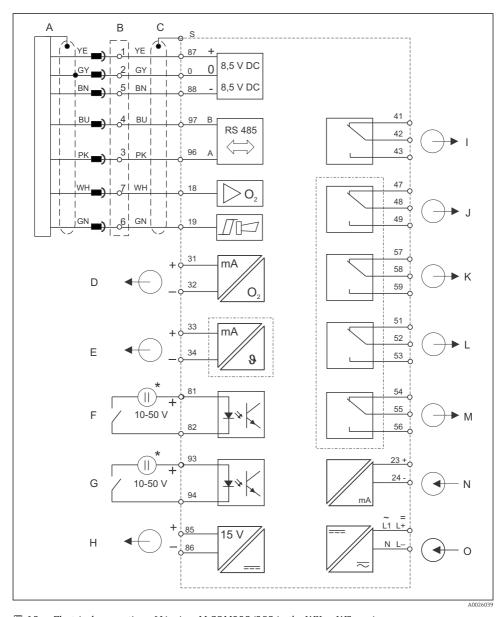
■ 10 Electrical connection of Liquisys M COM223/253 in the WX or WS version
