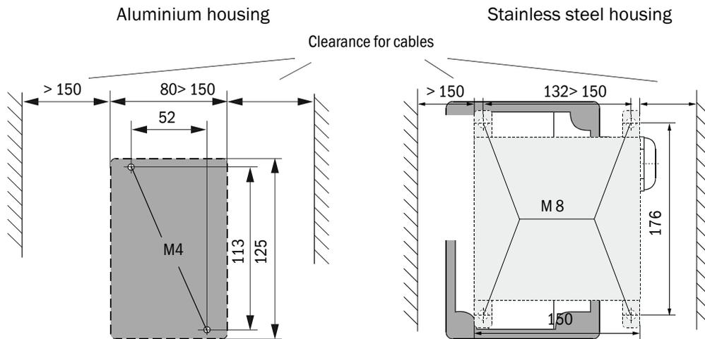
3.2.5 **Installing the temperature sensor of the temperature measurement option**
