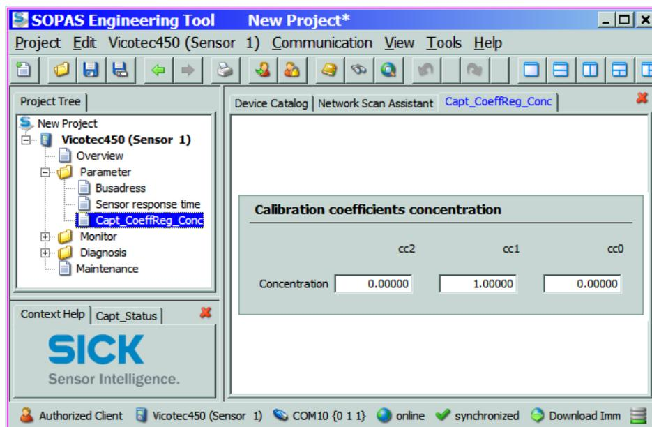
Switch the measuring unit back to "Measure" mode after entering the coefficients.
