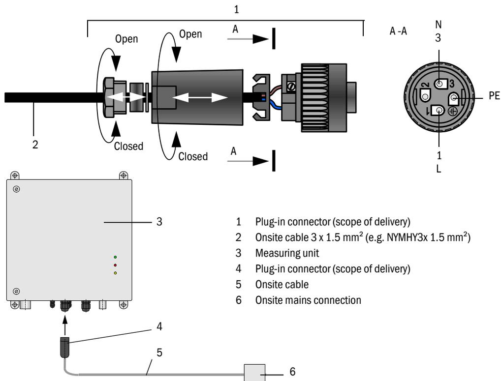
**Connecting the temperature measurement option**
