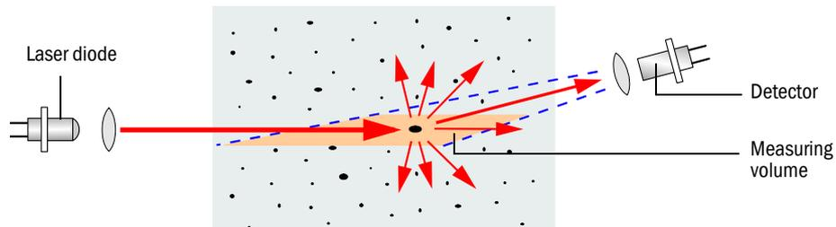
A laser diode beams the dust particles in the measuring air flow with modulated light in the visual range (wavelength approx. 650 nm). The light scattered by the particles is recorded by a highly sensitive detector, electrically amplified and passed to the measuring channel of a microprocessor as central part of the measuring, control and evaluation electronics. The measuring volume in the measuring cell is defined by the intersection between the transmitted beam and the receiver aperture.
