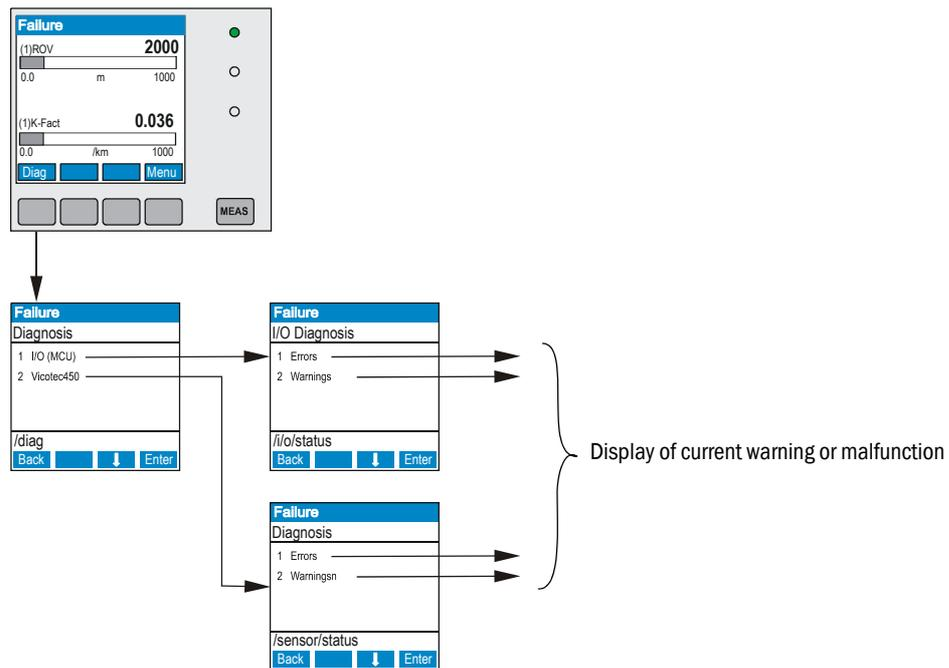
Detailed information on current device status is provided by the „Monitor/System state - details" (measuring unit) or "Diagnosis/Errors/Warnings" (MCU) directories.. Connect the measuring system to SOPAS ET and start the device file "Vicotec450" or "MCU" (→ p. 54, §4.1.3 and → p. 61, §4.1.4) to display the relevant information.
