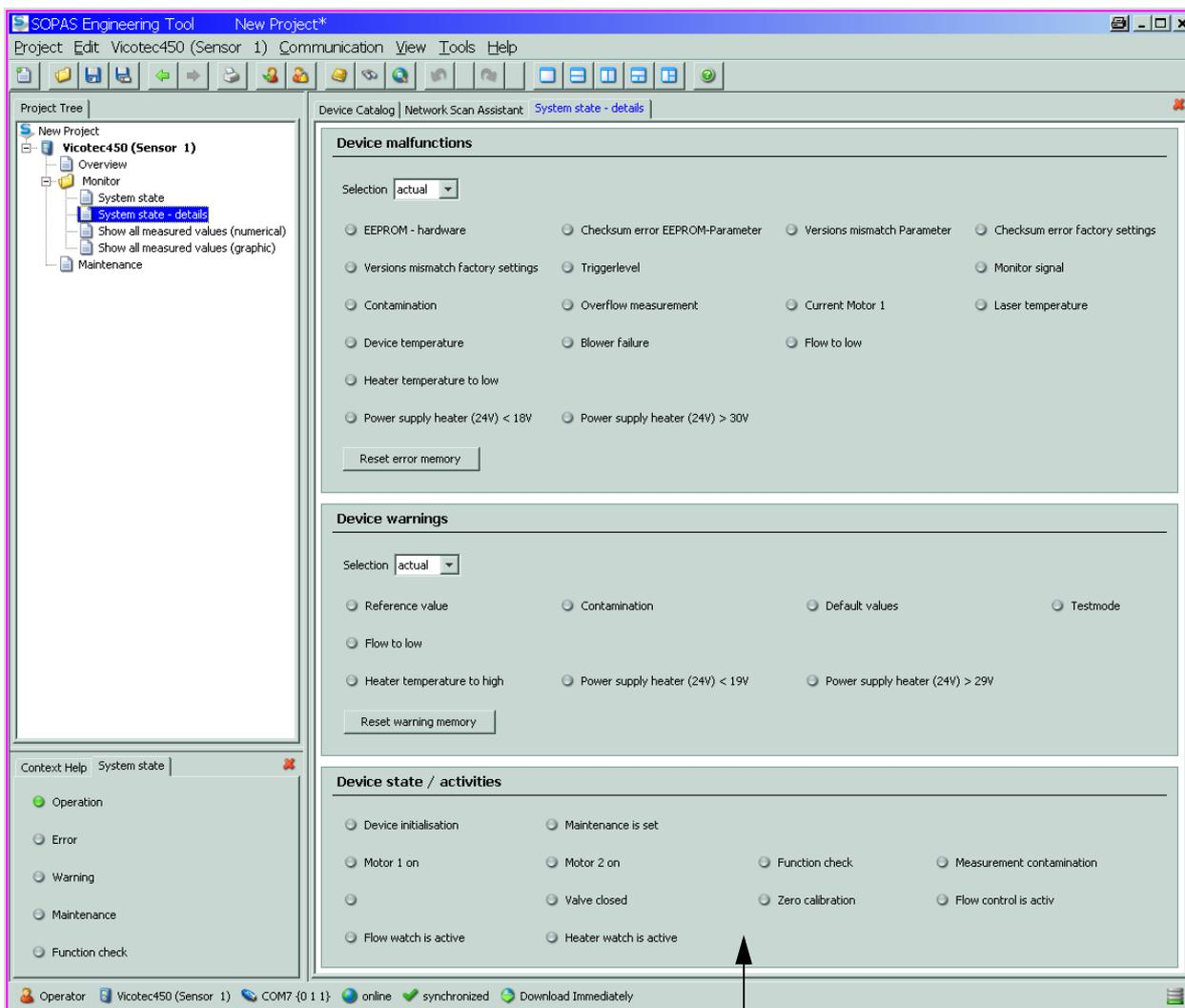
Current warning or error messages, or earlier messages stored in the error memory, can be shown by selecting "actual" or "memory" in the "Selection" window ("Device malfunction" group).→ p. 99, Fig. 87
