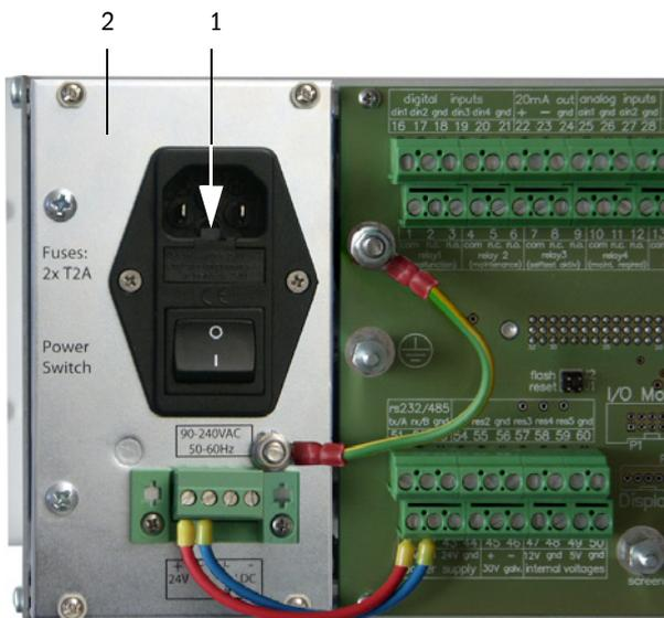
Power supply unit with terminal connection
