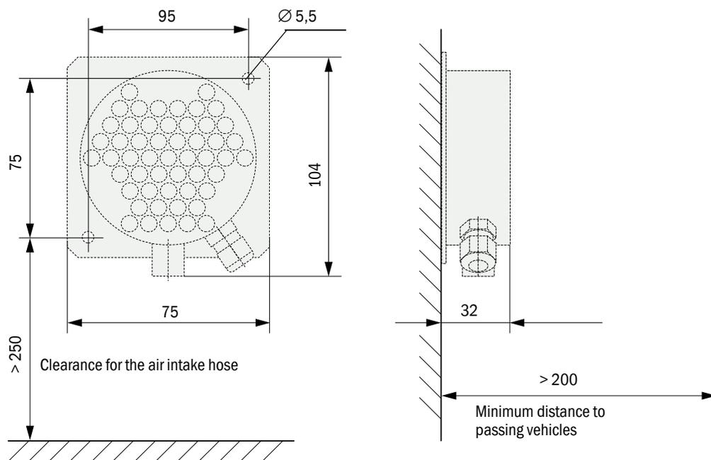
Figure 20 Installation dimensions for the air inlet with protective grating on the intermediate ceiling
