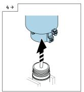
Carefully remove the housing from the sensor assembly, taking care not to damage the sensor cable.
