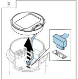
► Press the release mechanism and remove the display module.
