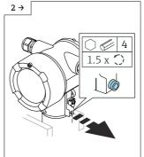
Housing lock for aluminum and stainless steel housing only.
