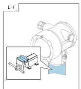
Protect the sensor assembly and housing from damage. Use a bench vise with braces.
