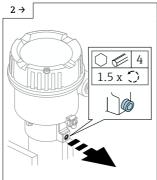
Housing lock for aluminum and stainless steel housing only. Not for plastic and hygienic housing.
