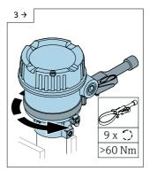
▶ Using a suitable tool, unscrew the housing by applying significant force (> 60 Nm). Place the gripping position below the cable entry. This involves applying force several times in and against the screw direction; the snap ring is intentionally destroyed in the process. Do not damage the coating of the housing.
