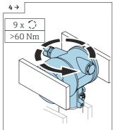
▶ Using a suitable tool, unscrew the housing by applying significant force (> 60 Nm). This involves applying force several times in and against the screw direction; the snap ring is intentionally destroyed in the process. Do not damage the coating of the housing.
