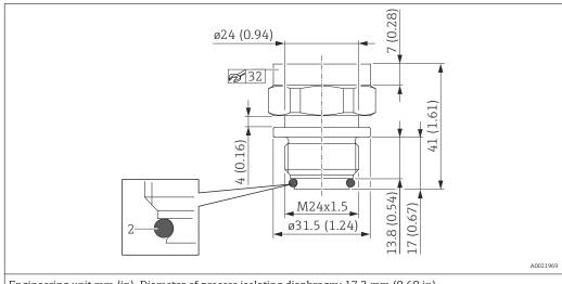
Engineering unit mm (in). Diameter of process isolating diaphragm: 17.2 mm (0.68 in)
