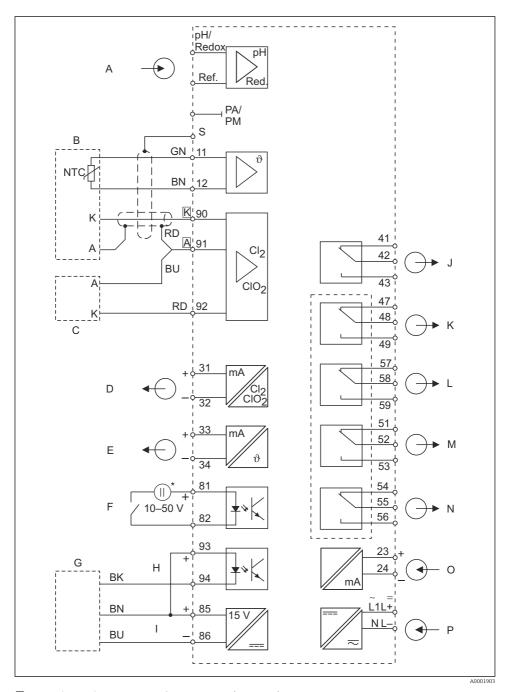
■ 7 Electrical connection of the transmitter (version 1)
