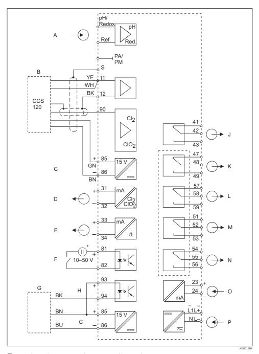
■ 8 Electrical connection of the transmitter (version 2)
