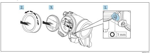
1. Loosen the securing clamp of the electronics compartment cover.
