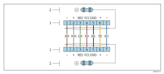
Terminals for connection compartment in the transmitter wall holder and the sensor connection housing
