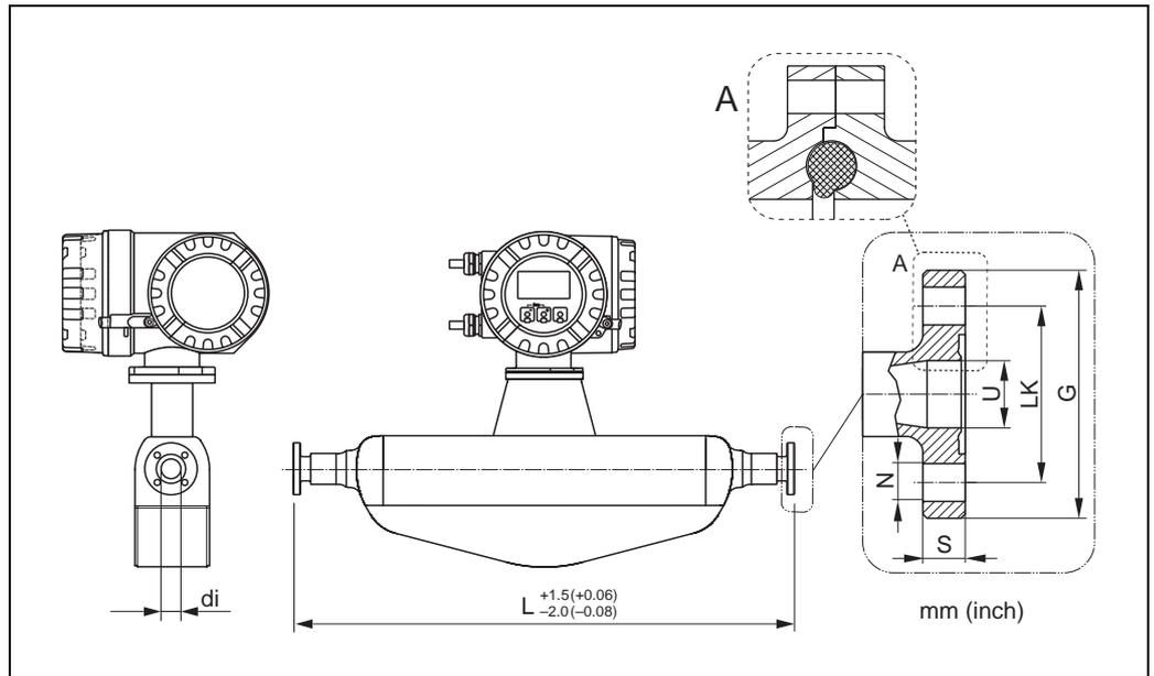
Detail A: The flange has the smaller groove for the O-ring on the sensor side. When mounting the sensor the corresponding flange must have accordingly a larger groove.
