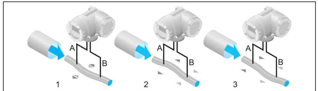
The phase difference (A-B) increases with increasing mass flow. Electrodynamic sensors register the tube oscillations at the inlet and outlet.
