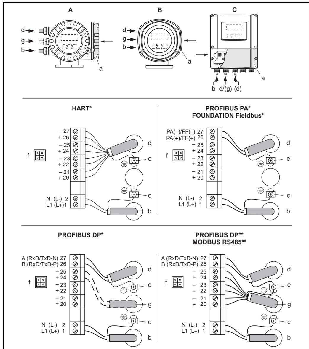
Connecting the transmitter, cable cross-section: max. 2.5 mm<sup>2</sup>
