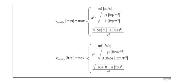
$v_{AmpMin}$  Minimum measurable flow velocity based on signal amplitude
