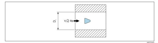
*D<sub>i</sub>* Internal diameter of measuring tube (corresponds to dimension K)
