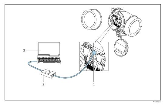
1 Service interface (CDI = Endress+Hauser Common Data Interface) of the measuring instrument
