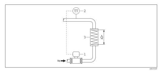
E 6 Layout for delta heat measurement of saturated steam and water
