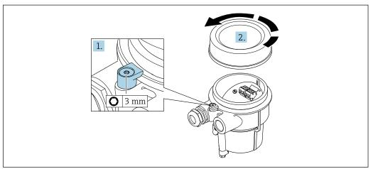
1. Loosen the securing clamp.
