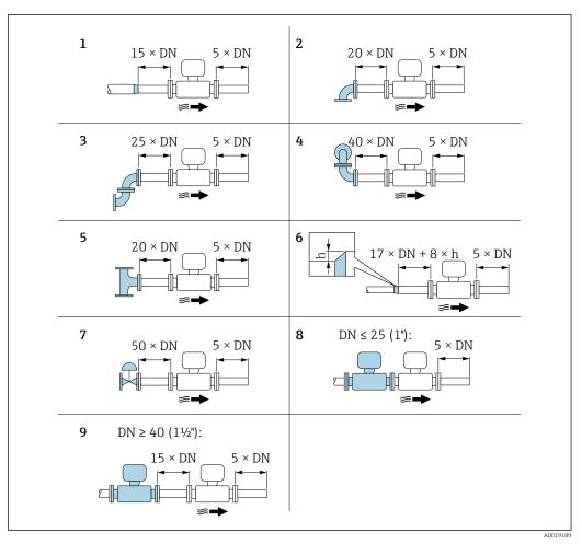
■ 5 Minimum inlet and outlet runs with various flow obstructions
