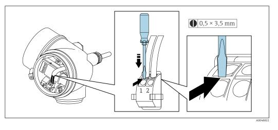
To remove a cable from the terminal, use a flat-blade screwdriver to push the slot between the two terminal holes while simultaneously pulling the cable end out of the terminal.
