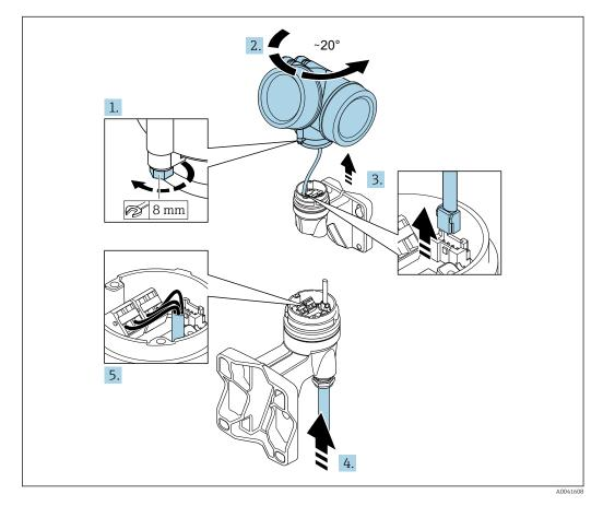
**1**. Loosen the securing clamp of the transmitter housing.
