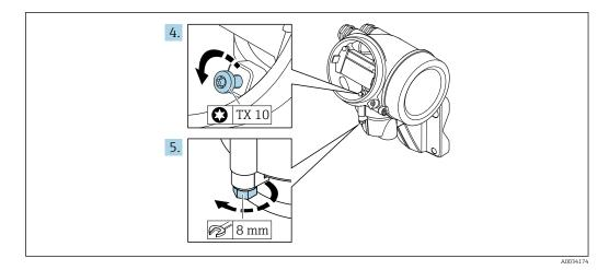
4. Loosen the locking screw of the transmitter housing.
