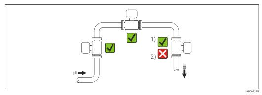
1 Installation suitable for gases and steam
