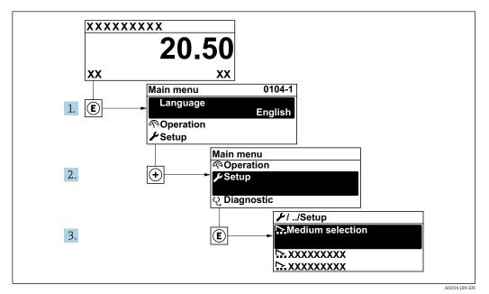
■ 20 Navigation to the "Setup" menuusing the example of the local display
