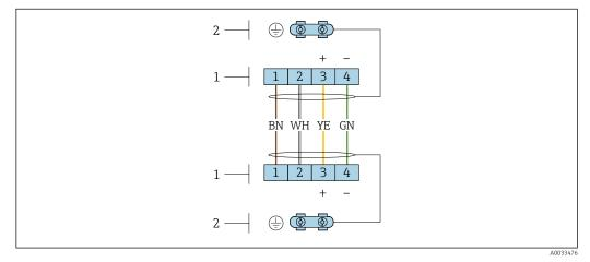
🗷 10 Terminals for connection compartment in the transmitter wall holder and the sensor connection housing
