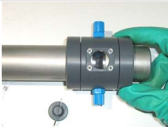
Figure 6 Turn the threaded rings loose -fitting on the threads
