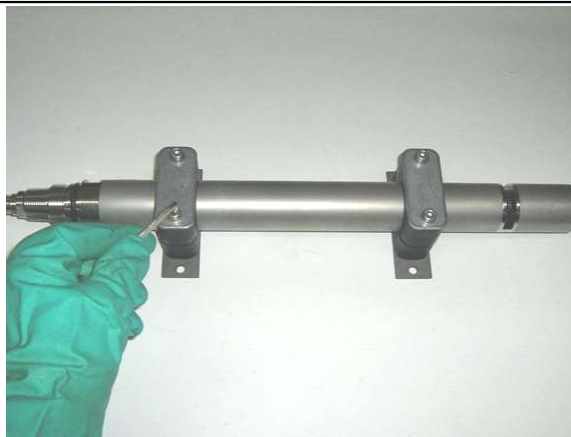
Figure 1 Mount the sensor CAS51D on the 2 holders
