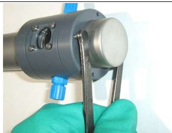
Figure 11 Loosen the threaded rings, using a face pin spanner
