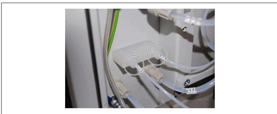
40 Coupling with short thread \frac{1}{8}'' \times 28\text{UNF} ETFE on condensate drain adapter for acid supply
