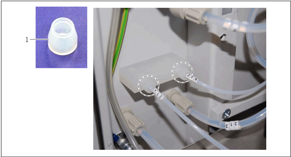
41 Cone for coupling \frac{1}{8} " \times 28UNF ETFE on condensate adapter for acid supply
