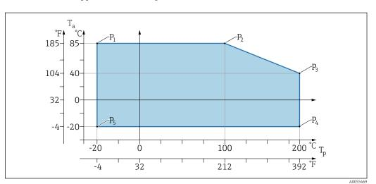
$\blacksquare$  7 Ambient temperature  $T_a$  depending on the process temperature  $T_p$
