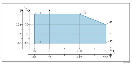
$\blacksquare$  5 Ambient temperature  $T_a$  depending on the process temperature  $T_p$
