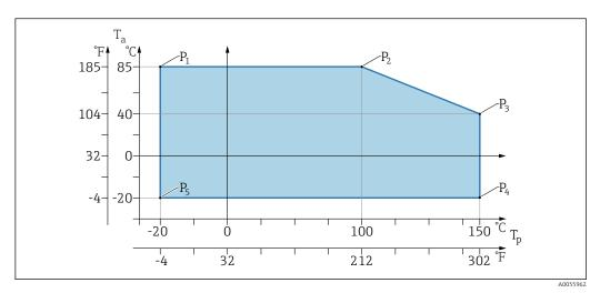
$\blacksquare$  6 Ambient temperature  $T_a$  depending on the process temperature  $T_p$
