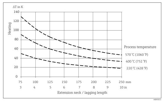
■ 10 Heating of the terminal head as a function of the process temperature. Temperature in terminal head = ambient temperature 20  $^{\circ}$ C (68  $^{\circ}$ F)+  $\Delta$ T
