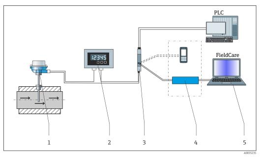
■ 1 Example of application, measuring point layout with additional Endress+Hauser components
