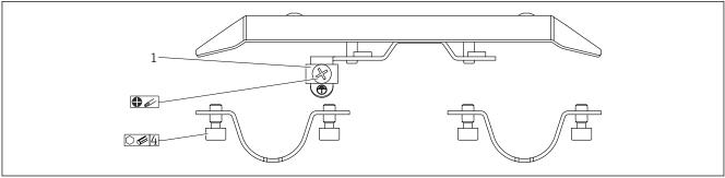
1 Ground terminal for connecting the potential matching line
