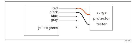
Resistance test diagram for HAW568-\*\*A\*\*4\*:
