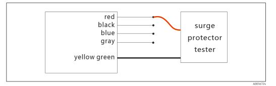
Breakdown voltage and reverse leakage test diagram for HAW568-\*\*B\*\*4\* and HAW568-\*\*A\*\*4\*:
