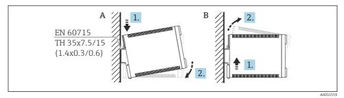
Mounting/disassembling the DIN rail housing. Unit of measurement mm (in)
