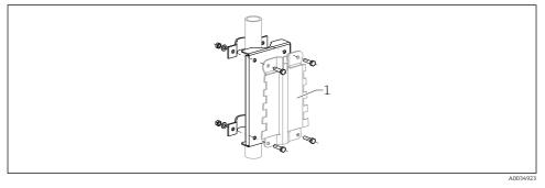
2 Mounting plate for mounting the polycarbonate field housing on a post
