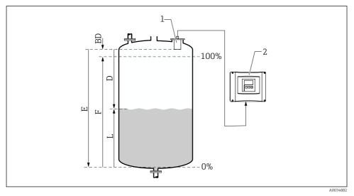
Empty and full calibration for level measurement
