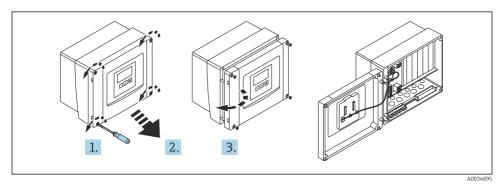
S Access to terminal compartment in polycarbonate field housing
