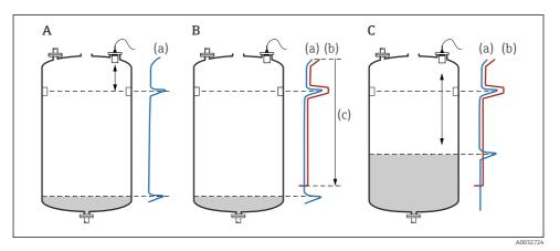
■ 12 Operating principle of the interference echo suppression (mapping) function
