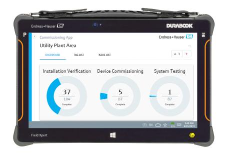
By integrating with Netilion, Endress+Hauser's cloud-based IIoT ecosystem, the team gained real-time access to device data, parameter configurations and verification reports. This eliminated the need to return to the office or docking station to organize documentation. Instead, commissioning data was saved and structured directly at the point of use, streamlining workflows and improving data accuracy.
