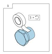
Only required if the lock screw is not pre-assembled with PTFE sealing tape.
