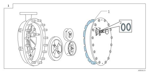
• Apply the PTFE paste to the supplied rear cover and O-rings.
