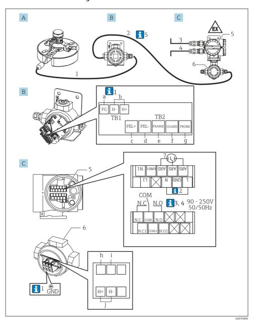
■ 16 Wiring of Ex d [ia] converter NRR261-5
