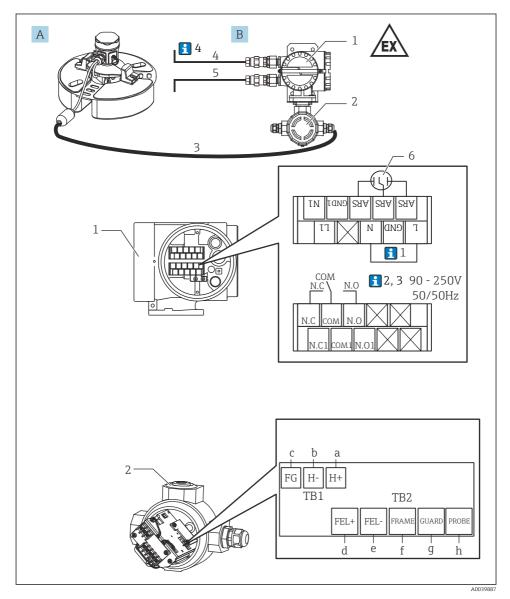
■ 14 Wiring of Ex d [ia] converter NRR261-4/A/B/C
