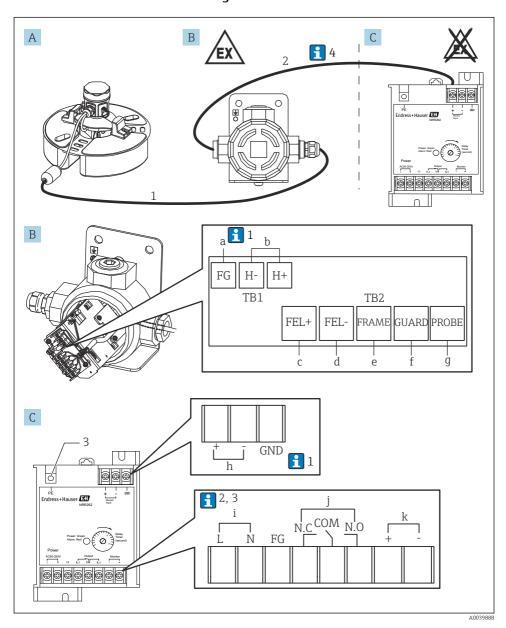
■ 15 Wiring of Ex [ia] converter NRR262-4/A/B/C
