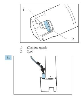
Connect the hose for the compressed air supply (to be provided on site) or compressor ( $\Rightarrow \square 31$ ) to the hose connection of the cleaning unit.
