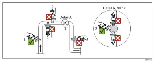
I1 Permissible and impermissible sensor installation positions with retractable assembly COA451
