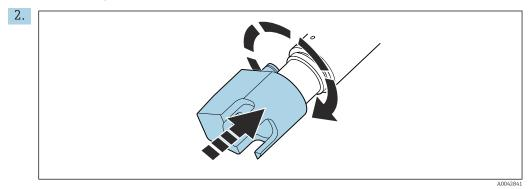
Screw on the cleaning unit or protection guard and tighten until the stop.
