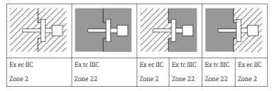
The device is designed for operation in explosive gas or explosive dust atmosphere as shown in the sketch above. In the event of potentially explosive gas-air and dust-air mixtures occurring simultaneously: Suitability requires further assessment.
