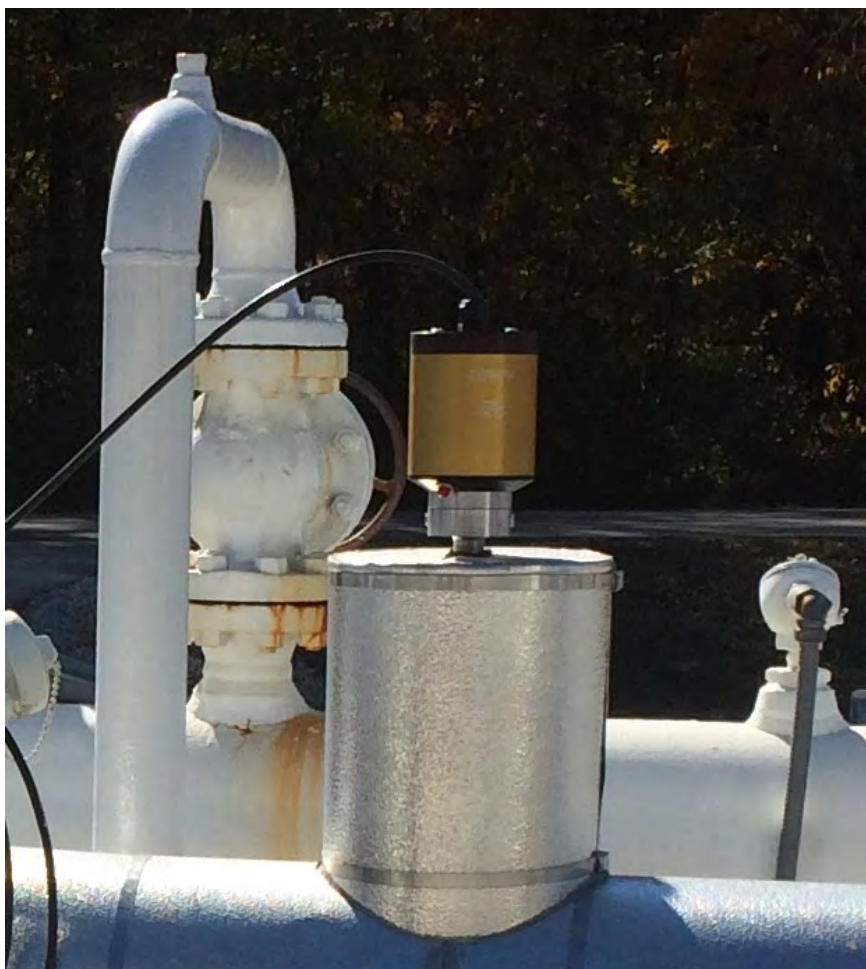
Raman Rxn-41 cryogenic probe
