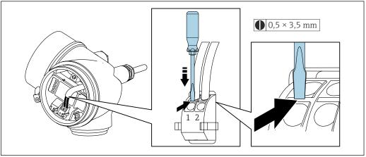
To remove a cable from the terminal, use a flat-blade screwdriver to push the slot between the two terminal holes while simultaneously pulling the cable end out of the terminal.
