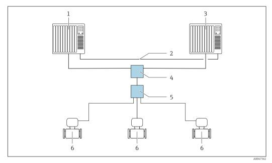
■ 17 Example of the layout of a redundant system (S2): star topology
