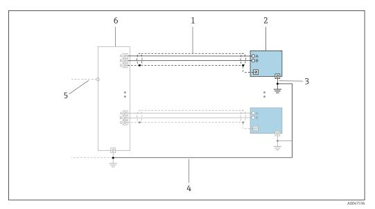
■ 9 Connection example for PROFINET over Ethernet-APL
