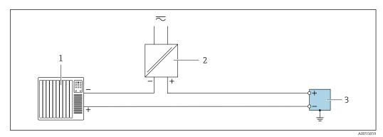
■ 7 Connection example for relay output
