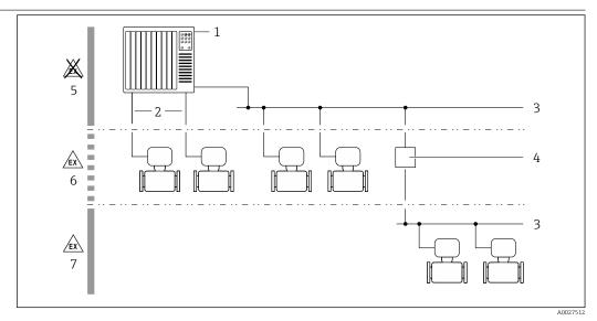
$\blacksquare 1$  Possibilities for integrating measuring instruments into a system
