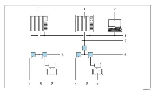
$\blacksquare$  45 Options for remote operation via FOUNDATION Fieldbus network
