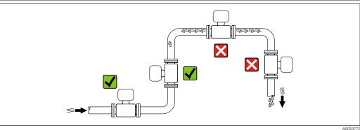
To avoid measurement errors caused by gas bubble formation in the measuring tube, avoid the following installation locations in the pipe:
