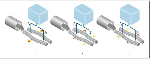
The phase shift (A-B) increases with increasing mass flow. Electrodynamic sensors register the tube oscillations at the inlet and outlet. System balance is ensured by the antiphase oscillation of the two measuring tubes. The measuring principle operates independently of temperature, pressure, viscosity, conductivity and flow profile.
